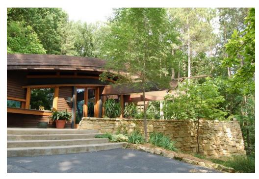
The house has curved walls and a curved roof matched with curved exterior beams laminated at the job site. It faces south and the large expanse of glass helps keep the living space comfotably warm. The home is fitted with a radiant heat system built into the tile floor.
